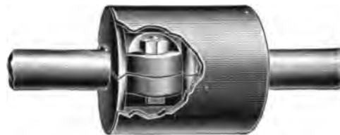
Fig. 5. Coupling with Tubular Shield.
